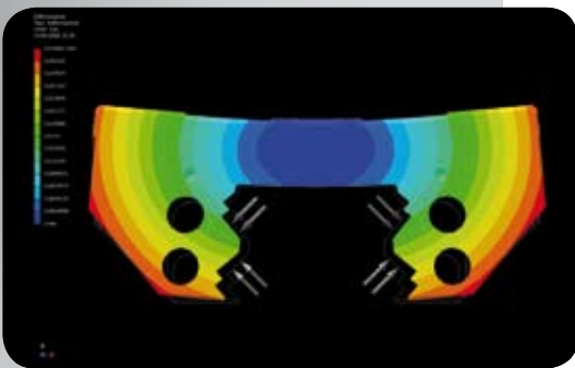
FEM-analyse of LC block
